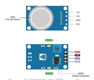
VCC: This pin powers the module, typically the operating voltage is +5V
